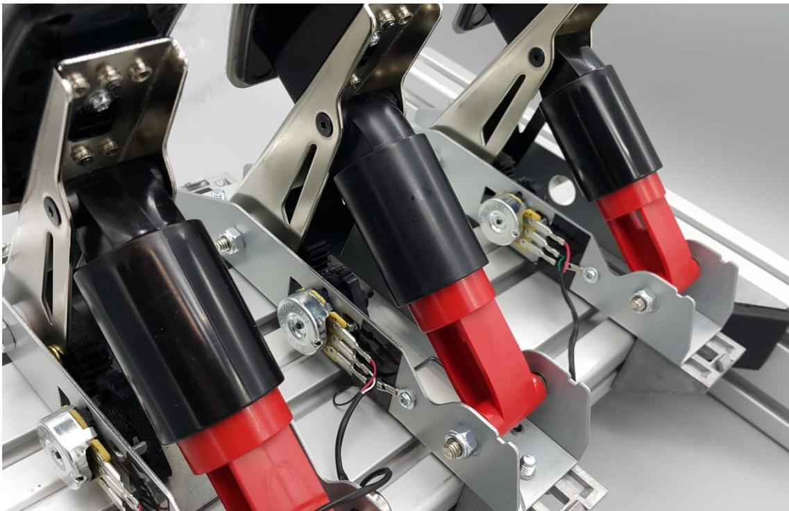
*Img 3.3.1: Aluminium profile 40 x 160mm, 350mm long. An example for a very stable mounting.*
