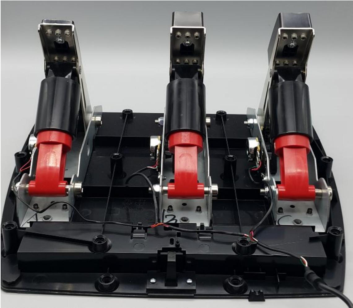
*Img 3.1.5: Almost there! The pedal-set with top case removed.*
