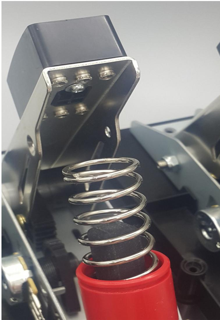
*Img 3.2.2: Original spring and rubber damper..*
